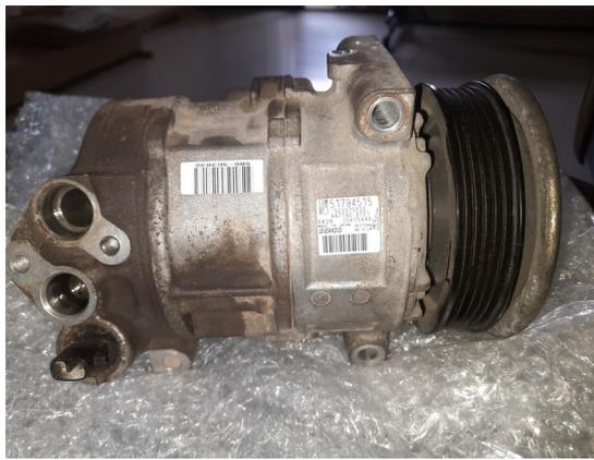
This is an a.c. compressor of Linea T-Jet 1.4 Petrol. Its par no. Is 51794515. Denso.
