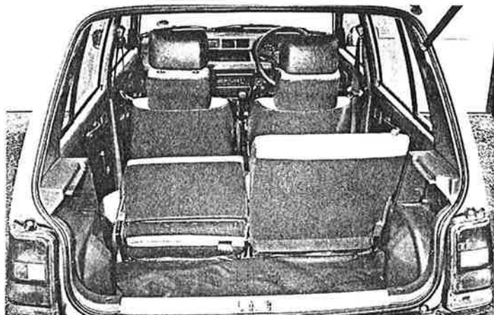
Domino's seat splits but only its backrest folds (above); Panda's bigger capacity can be further improved with a fully folding seat arrangement (below)
