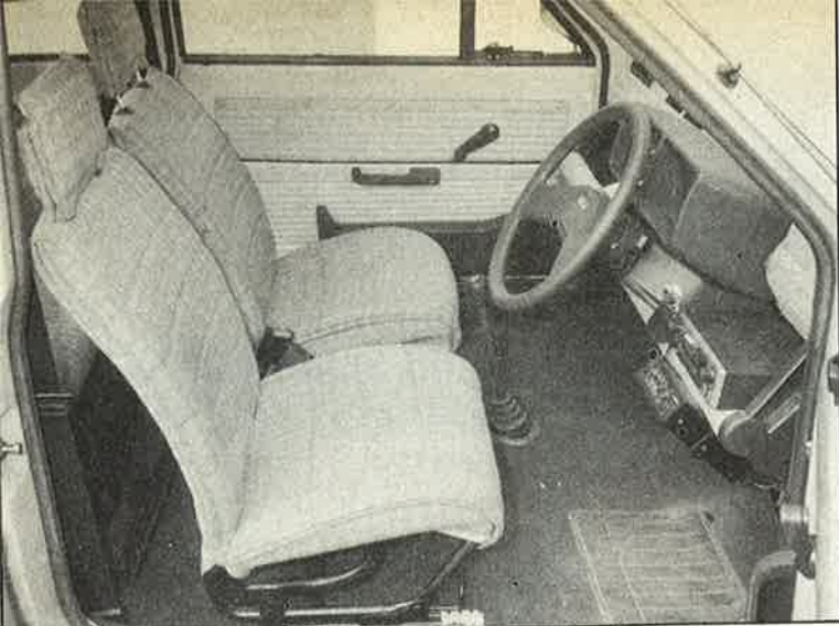
Slim front seats are more comfortable than they look. The stiff, metal release catch (below right) is not so clever, though, while the bar adjustment for the recline mechanism needs to be used with care
