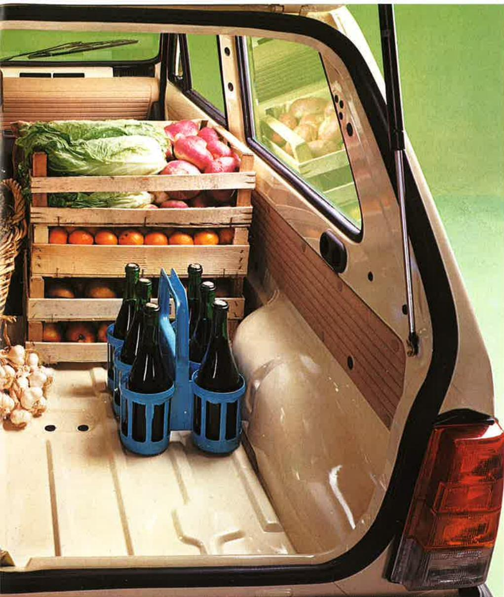
Have you noticed that the lower edge of the loading platform has a raised tailgate lip? This has the advantage of stopping a load from straining the door or breaking
