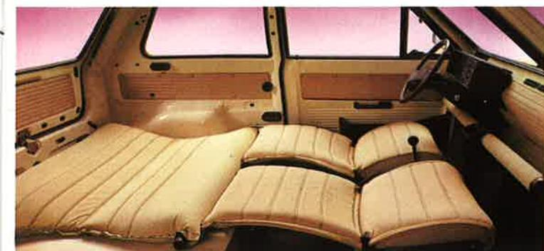
Another innovation is the ability to adjust the seats into a "bed" position by simply laying the rear seat over the load platform and fully reclining the front seat-backs (these are optionally available on the Panda 30, with removable head restraints).
