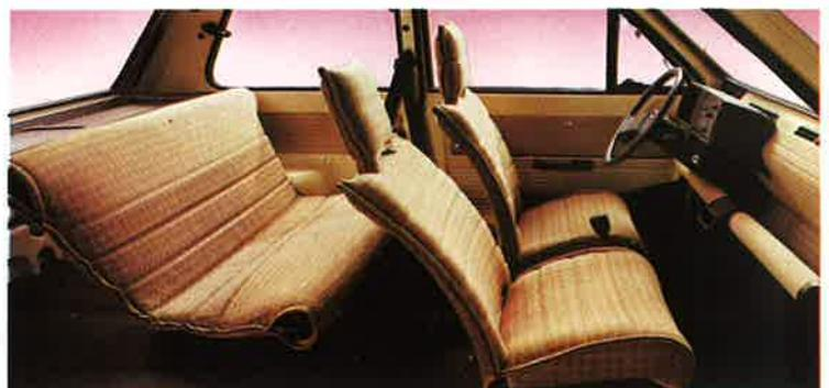
On the Panda 45, seats upholstered in cloth or leather-cloth; reclining front seats fitted with head restraints; pile carpeted floor and rubber mat in the rear.
